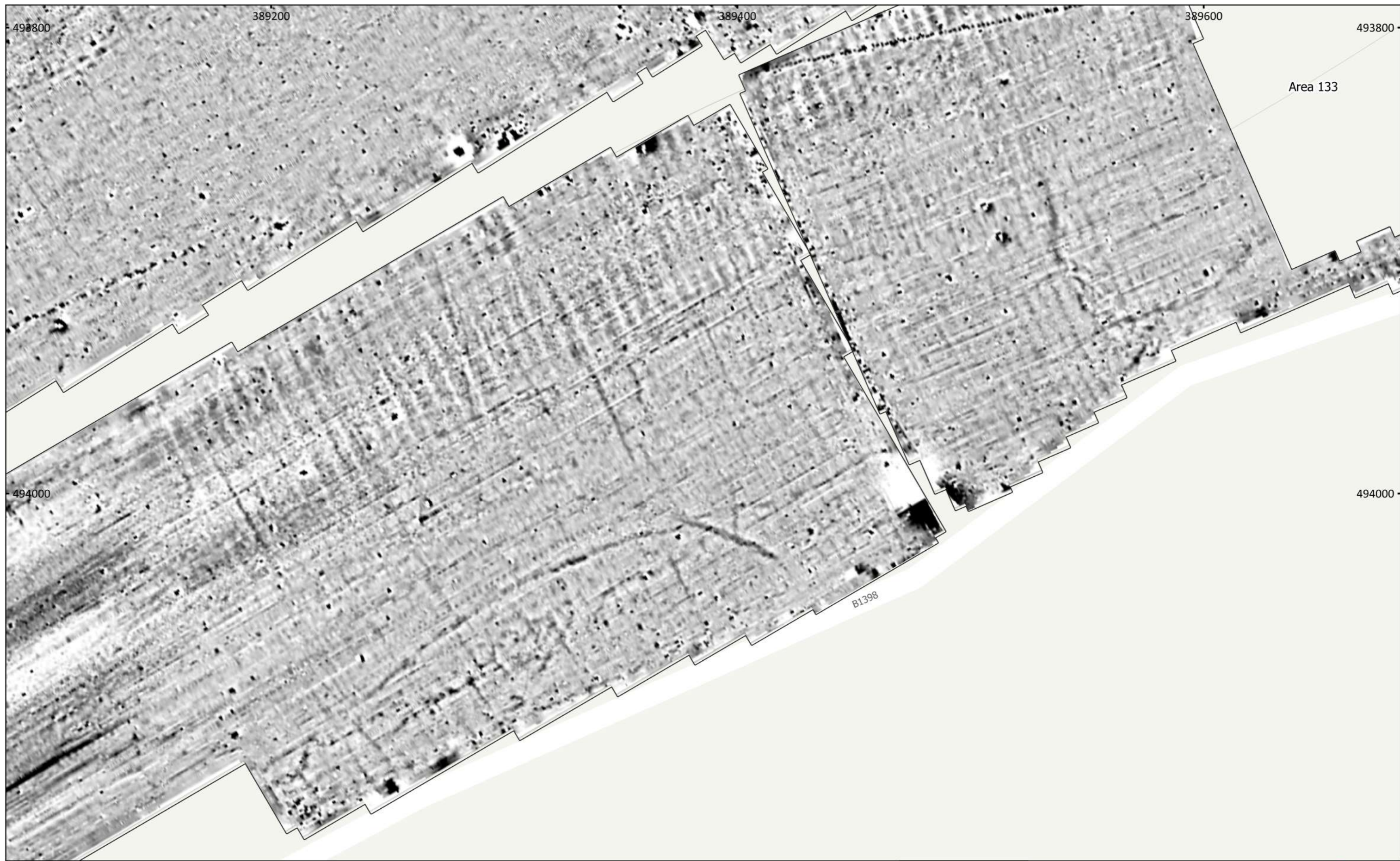
MSSK1393: Tillbridge Solar Scheme, Lincolnshire Figure 112 - Magnetic Gradient (Area of Archaeological Activity 5 (Areas 134 and 137)) 1:1,500 @ A3 Copyright Magnitude Surveys Ltd 2023 Contains Ordnance Survey data © Crown Copyright and database right 2023
